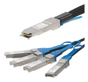
The QSFP4SFPPC3M is an MSA Compliant QSFP+ direct-attach Twinax breakout cable. It is designed, programmed and tested to bridge 40G network equipment with 10G compatible servers or routers. This passive Twin axial cable connects a single QSFP+ port to four 10G SFP+ ports and is fully hot-pluggable making upgrades and replacements seamless by minimizing network disruptions.
